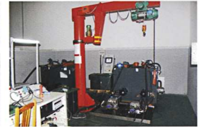
Power system integration testing station
