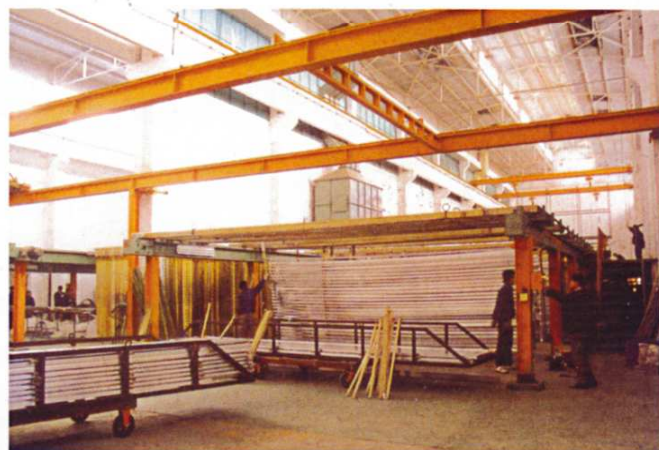
铝型材氧化着色生产线 Oxidation coating production line for aluminum shape material
