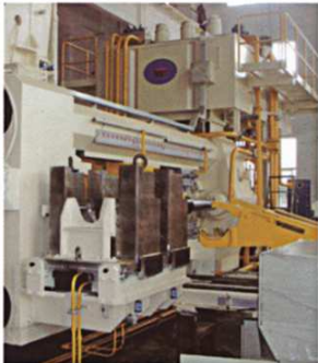
快速换模 Rapid mould changing
