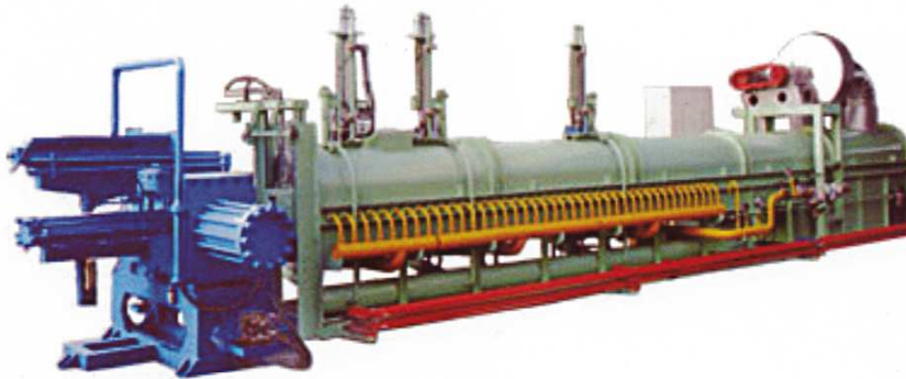
单棒快速带热剪炉 Single rod rapid hot shearing furnace
